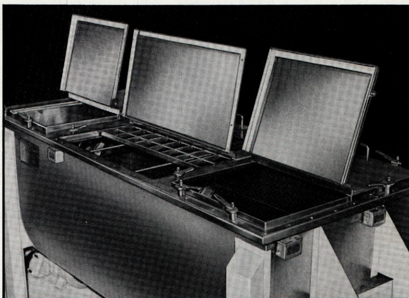
Two APS Model DRB-55 Sanitary Ribbon Blenders with low pressure heating jackets.
