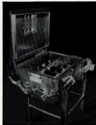
Model SRB-1000 Sanitary Blender with counter weighted cover for cheese blending/cooking.
